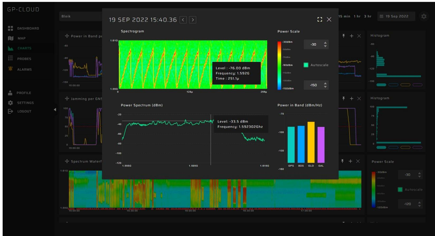
The GP-Probe TGE2 has an embedded RF signal analyzer with 60MHz real-time bandwidth and low noise figure < 3 dB. Every second, the signal analyzer acquires RF data and calculates power in band, power spectrum, and spectrogram for the most powerful events.
