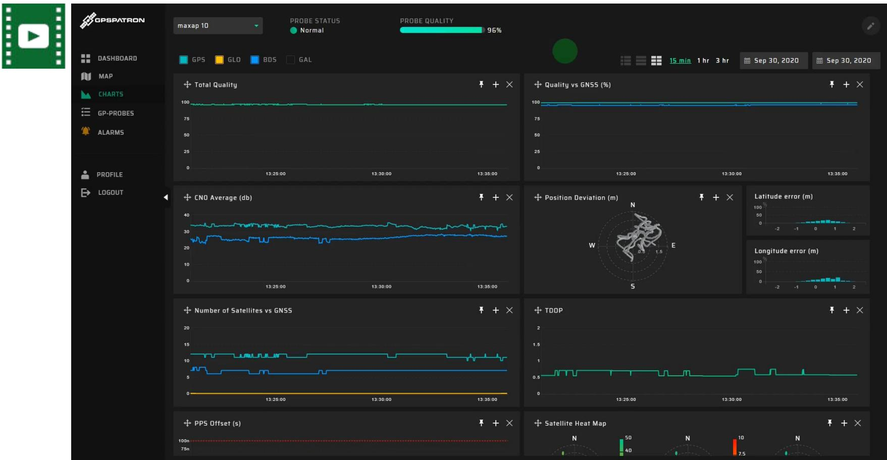
Every second, the GP-Probe measures many parameters of radio signals of all visible satellites: PR, CP, LockTime, Doppler, PR residual, CN0, etc. The GP-Cloud processes in real-time the data and estimates the quality/accuracy, and stores all results in the database.
